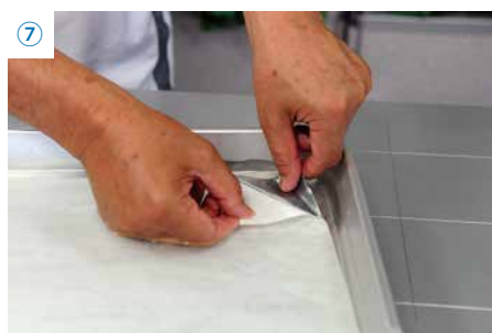
After soaking for a few minutes, the paper backing should peel off effortlessly from the film.
