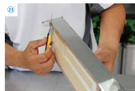
Cut excess film from the edges carefully while the model is still moist. When the film dries, it adheres to the surface of the clay with a paste. Once the film has dried, it becomes difficult to cut.
