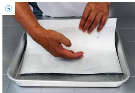
Having the paper face up makes it easy to confirm that the film is thoroughly soaked.
