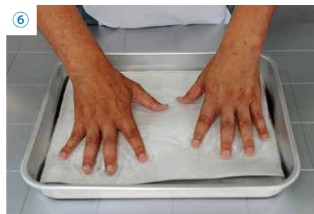
Completely submerge the film in water, applying gentle pressure to keep it beneath the surface of the water.
