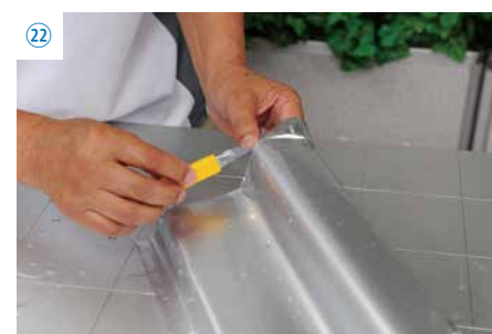
Cut excess film from the edges carefully while the model is still moist. When the film dries, it adheres to the surface of the clay with a paste. Once the film has dried, it becomes difficult to cut.
