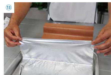
Moisten the surface of the clay by wetting it with water, then carefully apply the film to the model.
