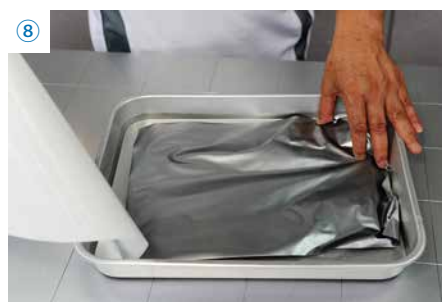
After soaking for a few minutes, the paper backing should peel off effortlessly from the film.
