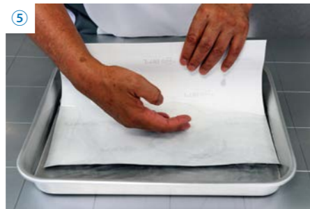
5 Having the paper face up makes it easy to confirm that the film is thoroughly soaked.
