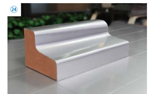
24 Finely finish the edges of the film with a spatula.
