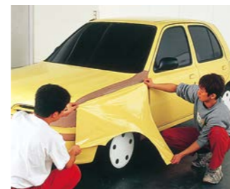
Example for use of Clay Modeling Film Clear *Yellow paint applied on Clear film.
