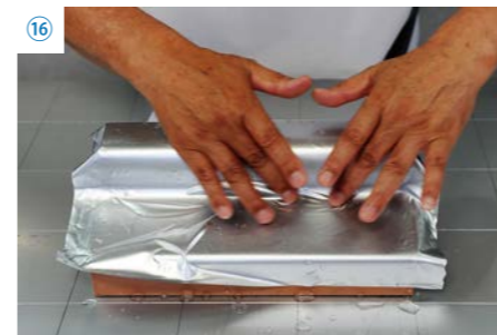
16 Adjust the film with a spatula to release water and air bubbles that appear on the surface, being careful to smooth corners. Finish by wiping away excess water with a cloth.
