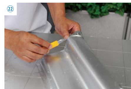
22 Cut excess film from the edges carefully while the model is still moist. When the film dries, it adheres to the surface of the clay with a paste. Once the film has dried, it becomes difficult to cut.
