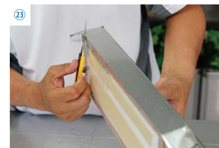
22 Cut excess film from the edges carefully while the model is still moist. When the film dries, it adheres to the surface of the clay with a paste. Once the film has dried, it becomes difficult to cut.
