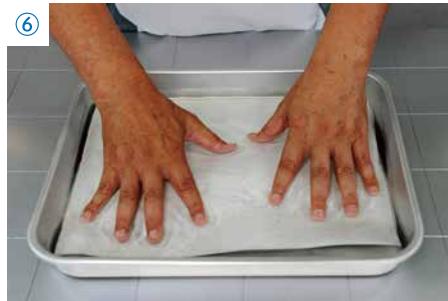
6 Completely submerge the film in water, applying gentle pressure to keep it beneath the surface of the water.
