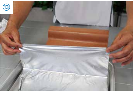
13 Moisten the surface of the clay by wetting it with water, then carefully apply the film to the model.
