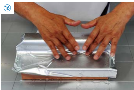
16 Adjust the film position, releasing of water and foam generated in the surface and clearance corner with a rubber spatula or squeegee, then it adhere to the surface and wipe away the water with a cloth.
