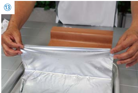
13 First moisten the surface of clay by spraying with water, then covering the film to the clay model carefully.
