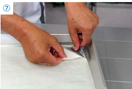
7 After soaking for a few minutes, the modelling film and absorbent backing paper will peel off easily either.
