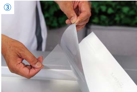
3 A protective film (clear polyester resin) is removed from the substrate film before first use.
